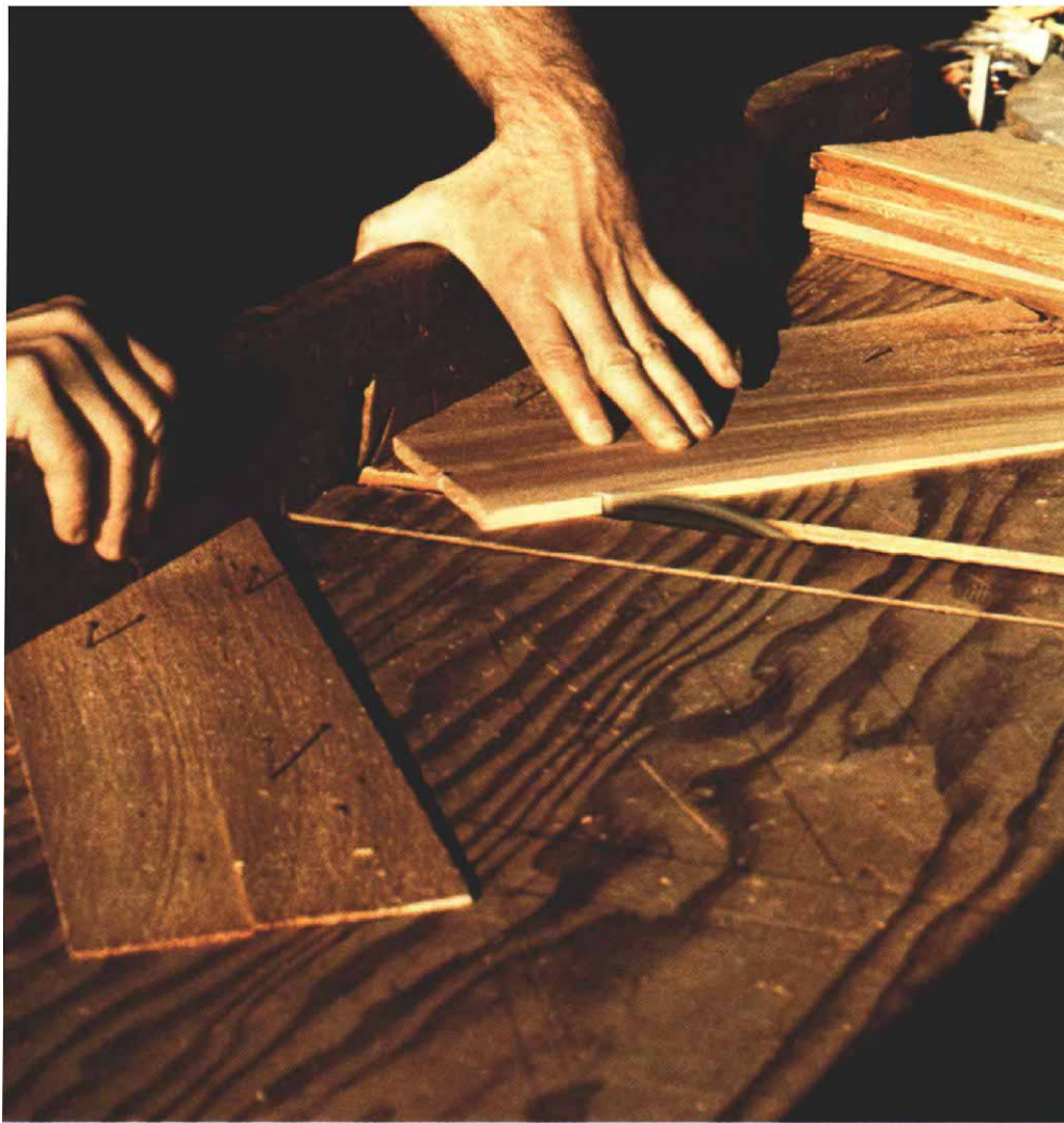
Cutting and fitting. A sliding-table jig for a table saw can make short work of cutting lots of shingles with diagonal points, such as the one being cut in the photo at left. Runners beneath the jig correspond to the grooves in the saw's table. The shingles are held against each tacked-on stop to register the cutting angle. Red cedar hearts emerge on the wall as the author places a row of shingles with half-circle cutouts over a row of pointed shingles (photo above). These decorative shingles are 5 in. wide, and they are centered over a row of square-cut shingles that are also 5 in. wide. Just above the shingles is a piece of 1x packing that trims the top of the wall.
